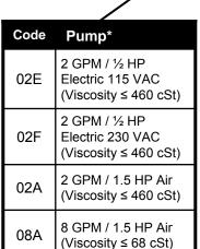
Performance will vary depending on temperature, filter combination, bypass options, hose sizes, connectors, and fluid type.
