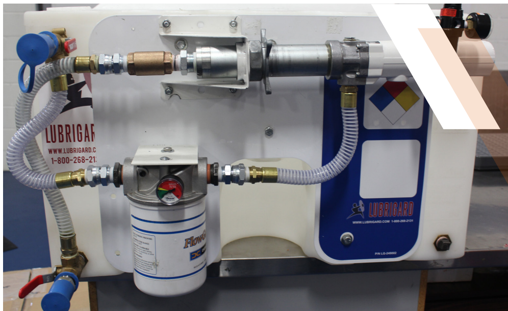
FIG.4F1. POLY TANK COMPLETE WITH PUMP, FILTER, HOSES, VALVES AND QUICK CONNECTS.
