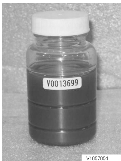
Fig.2 Oil-sample bottle with attached label
