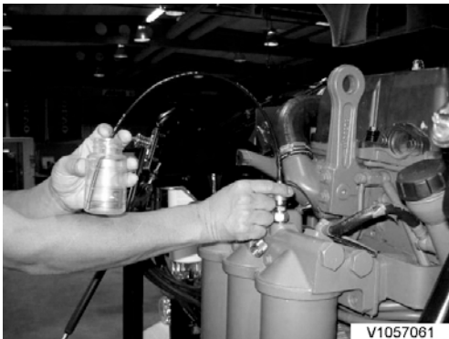
Fig.9 Example of sampling method with hose
