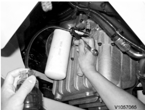
Fig.12 Example of sampling method with quick-action coupling
