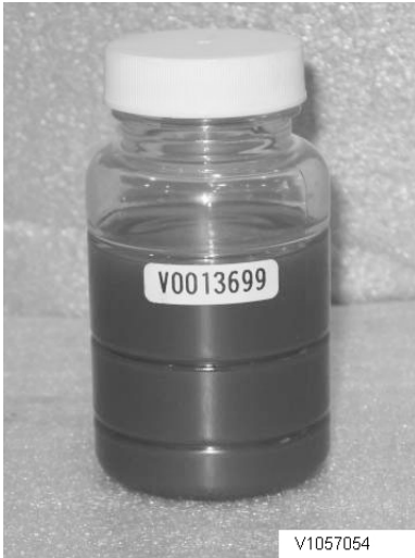
Fig.2 Oil-sample bottle with attached label
