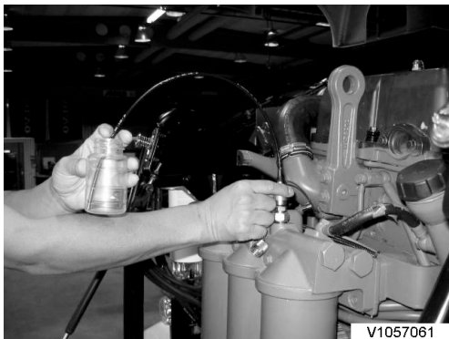
Fig.9 Example of sampling method with hose
