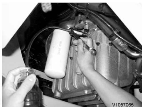
Fig.12 Example of sampling method with quick-action coupling
