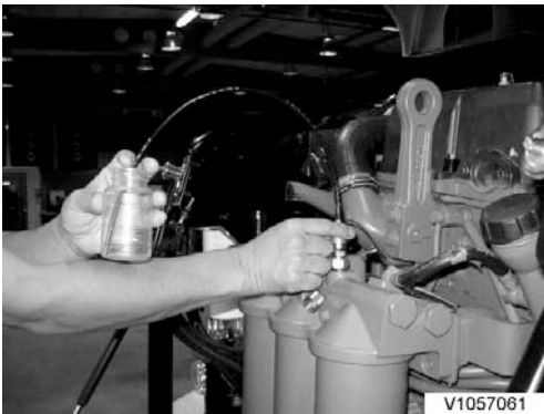
Fig.9 Example of sampling method with hose
