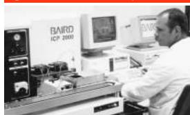
s pectrometric, or SOAP, analysis is the foundation of any monitoring system. SOAP measures concentrations of the shear mixed layer wear particles present in the oil. Trendline analysis of this data detects subtle changes to wear modes in the system, usually long before any significant wear to those components occurs.
