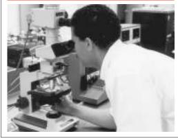
A ny indication of abnormal wear, either by DR-Ferr or SOAP analysis, will trigger an Analytical Ferrogram (A-Ferr). A sample of the microscopic wear metals, and contaminants present in the oil, are deposited on a slide and examined under a high-powered microscope. By analyzing particle morphology, A-Ferr indicates the mode(s) of wear present in the system, and can detect the cause(s) of abnormal wear modes.
