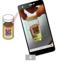
Scan the sample bottle label from your oil sample for the selected machine and component.
