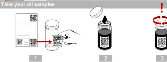
Remove the sample label from the sample form and stick to the sample bottle. Take the oil sample as you normally would and re-cap the sample bottle.
