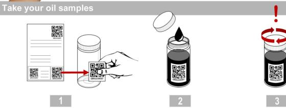
Remove the sample label from the sample form and stick to the sample bottle.
