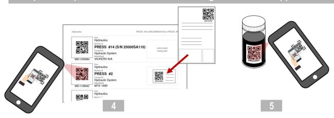
Using the app, scan the QR code of the machine the sample was taken from. Remove the tracking label from the sample form and stick to the asset log booklet.
