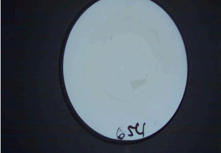
MPC (Varnish Test)
