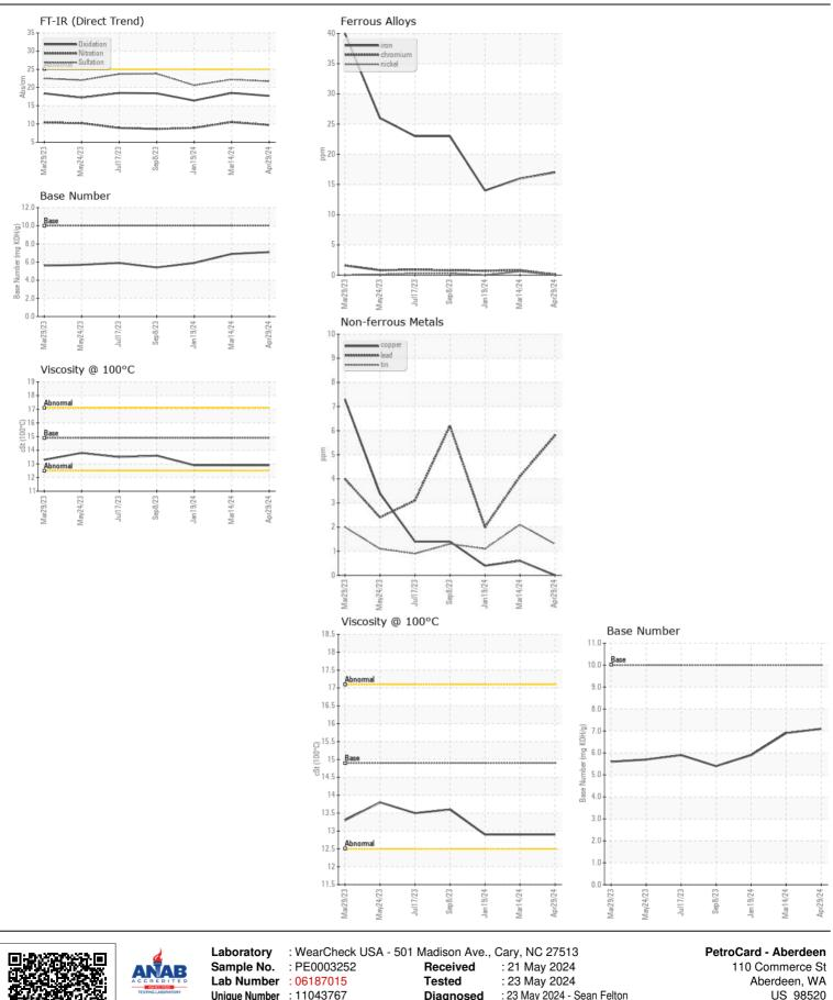
Unique Number : 11043767 : 23 May 2024 - Sean Felton Diagnosed Test Package : CONST (Additional Tests: FT-IR, ICP, KV100, SCREEN, TBN) Certificate L2367 To discuss this sample report, contact Customer Service at 1-800-237-1369. smcnealley@petrocard.com \* - Denotes test methods that are outside of the ISO 17025 scope of accreditation. Statements of conformity to specifications are based on the simple acceptance decision rule (JCGM 106:2012)
