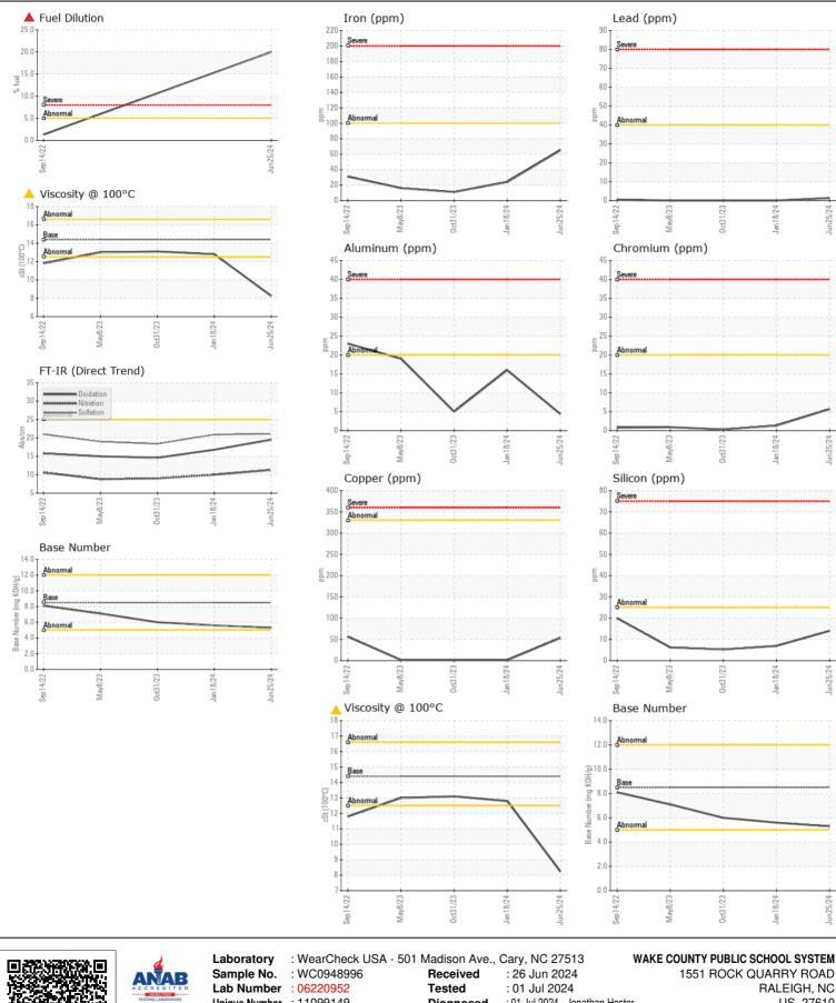
Unique Number : 11099149 Diagnosed : 01 Jul 2024 - Jonathan Hester Test Package : MOB 1 (Additional Tests: FuelDilution, PercentFuel, TBN) Contact: DEVIN WEBER Certificate L2367 To discuss this sample report, contact Customer Service at 1-800-237-1369. \* - Denotes test methods that are outside of the ISO 17025 scope of accreditation. Statements of conformity to specifications are based on the simple acceptance decision rule (JCGM 106:2012)
