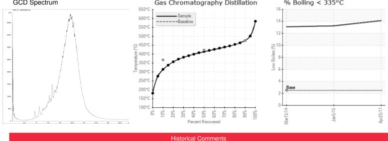
There is an indication of thermal cracking as the oil seems to have abnormall high light ends. If it is possible to vent the light ends out of the system through the expansion tank, then I would suggest that this be done. I would suggest tha we re-sample the oil in this unit. It is about the same as the sample from 3/5/2014 01/05/15 (GCD) 10% Distillation Point is severely low. (GCD) % < 335°C is abnormally high. COC Flash Point is abnormally low.
