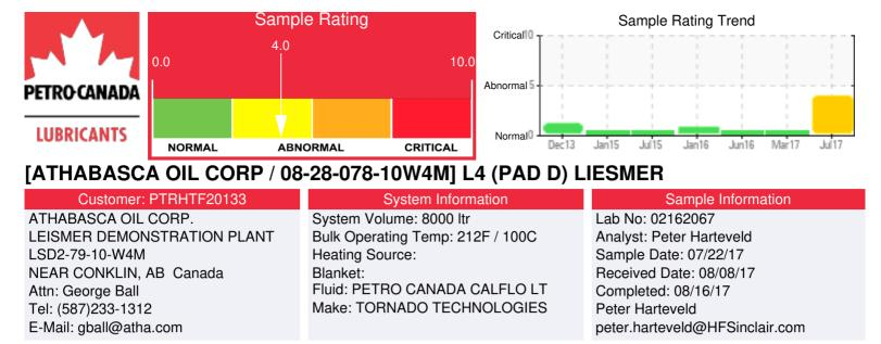
Recommendation: The fluid is in a good condition and suitable for further use. The analysis does show indications of degradation. The % boil-off <335C is elevated and the 90% GCD temperature is high. It is recommended to vent off low boiler vapors to atmosphere on a regular basis. (once per month) Please re-sample in 12 months and list fluid service life when sending in the sample.
