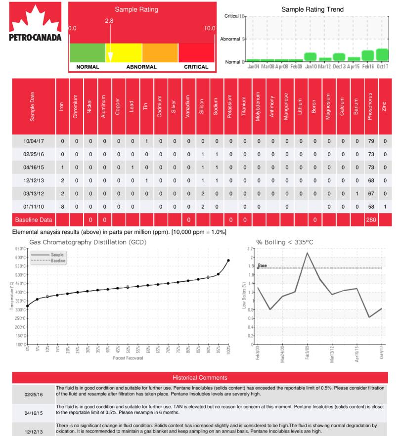
The oil condition looks very similar to previous samples. There has been a slight thickening of the fluid but tests for oxidation do not seem to indicate major 03/13/12 degradation. Keep sampling every year at least.
