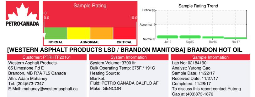
Recommendation: The current fluid is in good conditions and suitable for further operation. Please take one sample in one year and monitor the conditions. Please also provide the oil working hours with the next sample.
