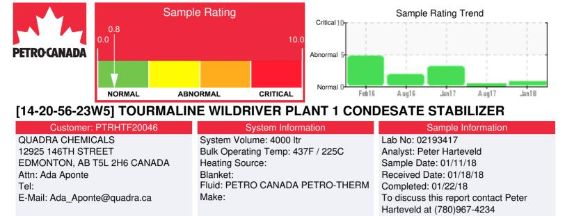
Recommendation: Please fill in service life of the fluid. This is required for interpretation of the analysis. The fluid shows early signs of thermal degradation but is still in a good condition and suitable for further use. Please re-sample in 6 months.
