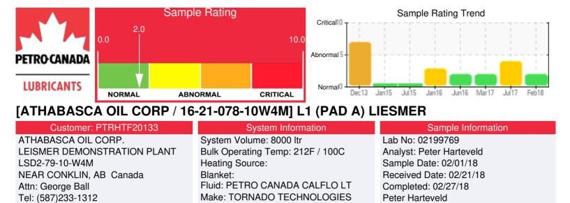
Recommendation: The fluid is in good condition and suitable for further use. Low boiler vapor content is high (GCD% <335C = 48.72%). For fresh Calflo LT this is 35%. This is a result of normal thermal degradation of the fluid and can be rectified by venting low boiler vapor to atmosphere. Please re-sample in 6 months.
