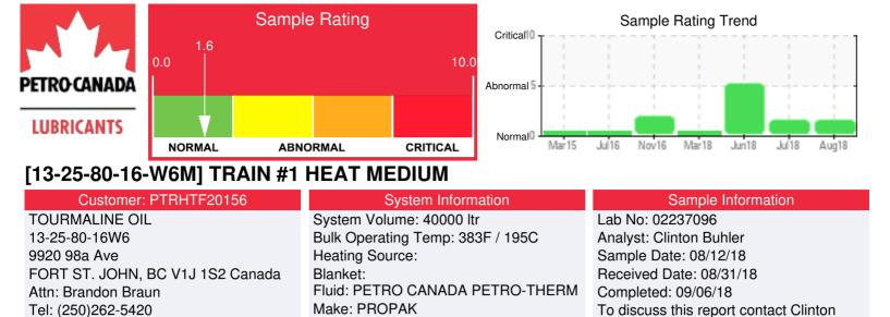
Recommendation: Flash Point is severely low. Low flash point is a safety concern. % boil-off has increased to 6.27% from 2.42%. This may be attributed to either the condensate contamination and/or thermal degradation. This should be less than 1. Viscosity remains low; currently at 25 cSt vs 34 cSt of new fluid. Consider fluid replacement as the safest method to bring flash point back to acceptable values. Re-sample once fluid has been restored.
