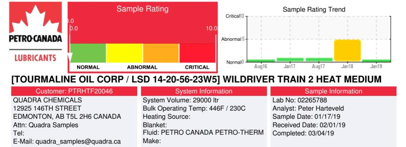
Recommendation: The fluid is in a good condition and suitable for further use. Please re-sample in 12 months.
