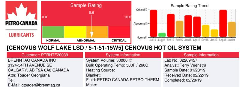
Recommendation: GDC 10% Distillation as well has the Flash Point are low indicating some lighter ends. Venting of the system is required. Vent lighter ends off system and resample in 6 months.
