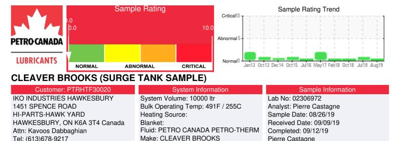
Recommendation: We can see a very small trace of bitunem in the sample. The oil, is OK for continuous use, resample at the next sample date.
