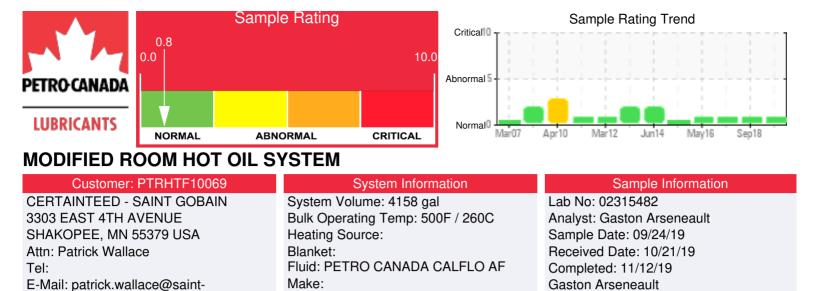
Recommendation: The oil is holding steady with the properties remaining normal from sample to sample. Contamination by asphalt, water or other elements is insignificant or non-detectable. No actions needed at this time. Re-sample at next scheduled interval
