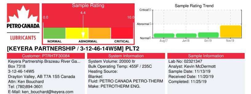
Recommendation: The very low flash point combined with low viscosity are symptoms of thermal cracking, but given the history of this system likely from a prior exchanger leak. Fortunately these low valves are not significantly worsening since previous sample. Suggest submitting annual samples or sooner if fluid becomes stressed or if exchanger leak is suspected.
