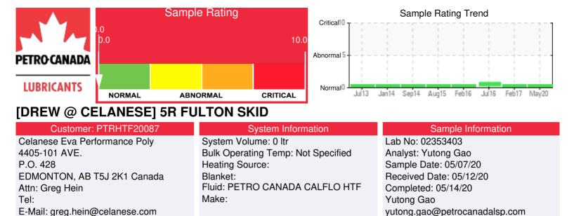
Recommendation: The current fluid has a very similar condition as the sample in 2017. The oil viscosity and flash point are normal. There is minimum oxidation or water contamination. It is suitable for further use. Please take one sample in 18 months to monitor the conditions.
