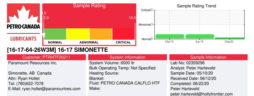
Recommendation: The fluid is in a good condition and suitable for further use. Viscosity is slightly high. This combined with elevated distillation temperatures indicates that the fill contains a heavier fluid, possibly Sunoil 21. This is not a problem. Please re-sample in 12 months.
