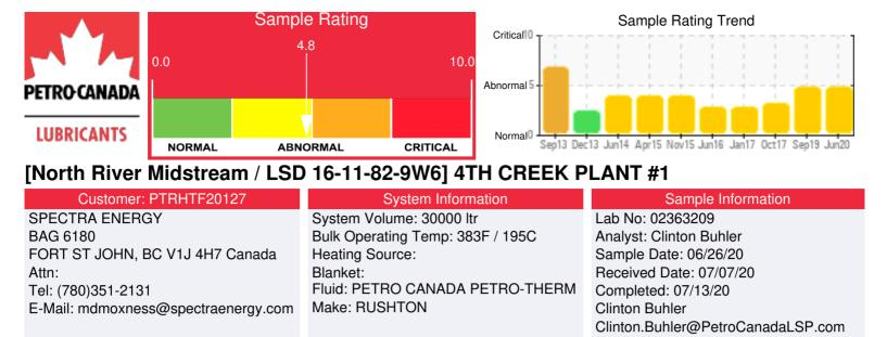
Recommendation: Sample results indicate that fluid degradation and system fouling is ongoing: Solids has increased to 2.23%, acid number is at 1.02 and is well above the threshold of 0.4% for when sweetening would have been of value. % of low boiling vapors (3.21%) also indicates thermal degradation ongoing along with the oxidation.System cleaning and fluid replacement is recommended.
