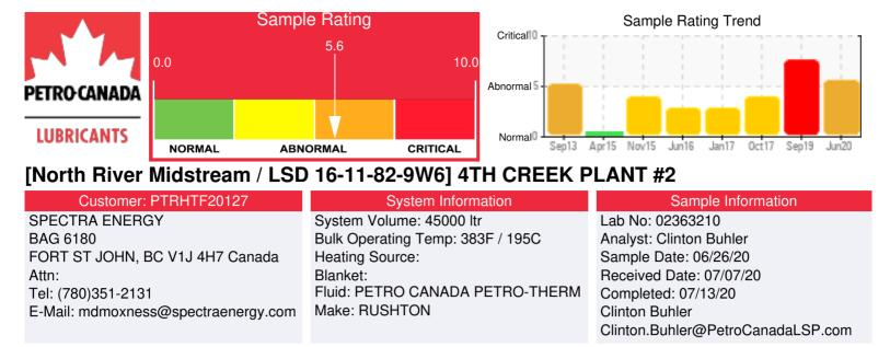
Recommendation: Sample results indicate continued system fouling as Solids content has increased from 1.92% to 4%. The fluid's acidity (AN) has increased to 1.19 along with elevated viscosity at 60.9 cSt indicates oxidation degradation. It is recommended to perform a system cleaning and fluid replacement before conditions degrade even further.
