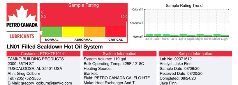
Recommendation: GCD 10% distillation point has improved from last sample. Oil appears to be in great condition and is suitable for continued use. Please resubmit sample for testing in one year.
