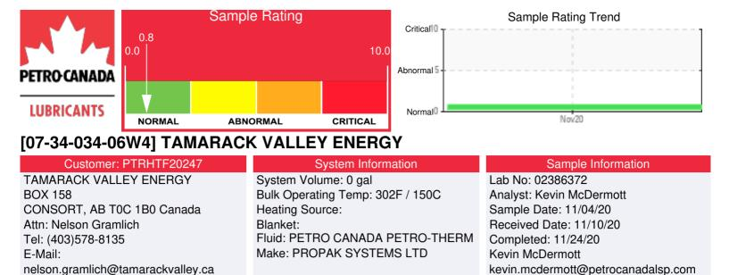
Recommendation: Fluid is in good condition overall. Ensure blanket gas is always maintained to prevent oxidation. Suggest submitting samples annually to proactively monitor fluid condition.
