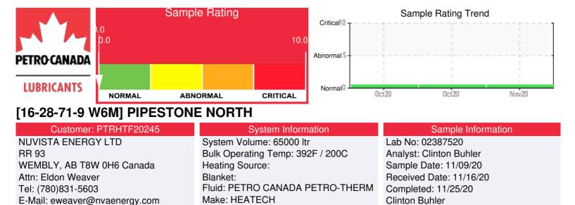
Recommendation: Final sample of the fluid after filtering has been completed. ISO particle count remains at 23/21/14 yet solids has gone from 0.069% to 0.046% which is also an indication of efficient filtering. Please re-sample once system is operational at normal operating temperatures.
