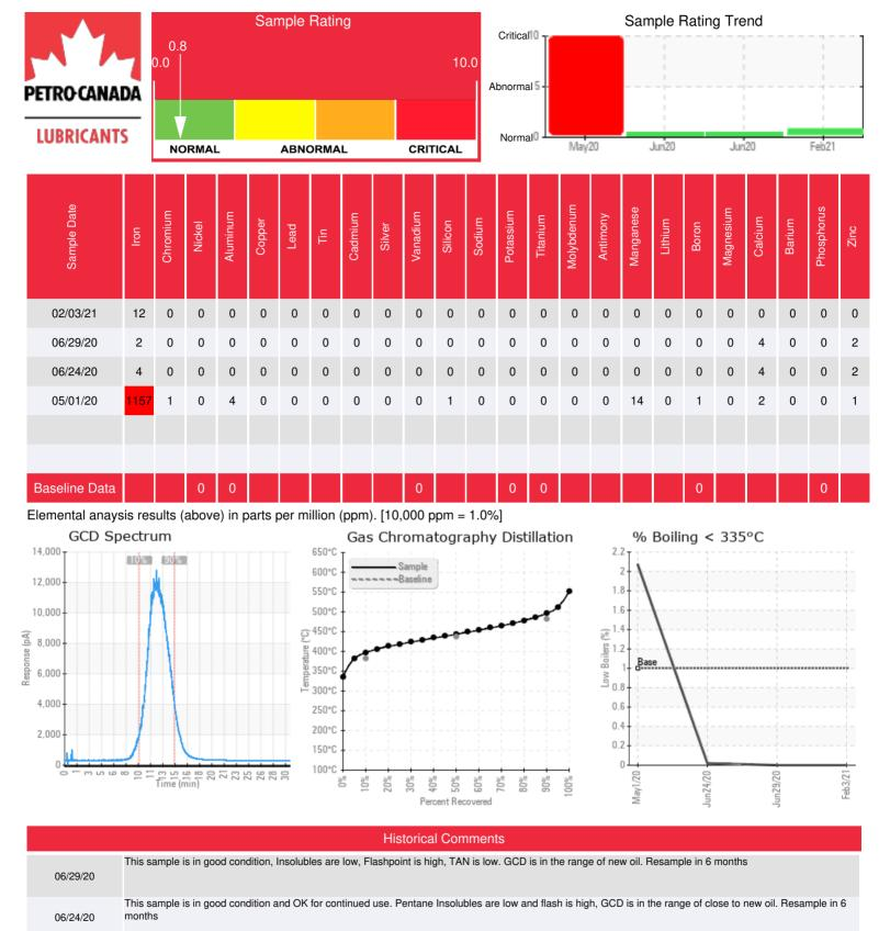
Fluid is in very poor condition due to severe oxidation. Very high iron content indicates corrosion. The Acid Number, viscosity and solids content also all 05/01/20 extremely high. System will require internal cleaning and fluid replacement.
