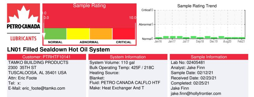
Recommendation: While the color of this sample is darker and not consistent with previous samples from this unit, the test data shows that the fluid is in good condition and is suitable for continued use. Please resample and submit for testing in one year. Please also remember to include the oil age on future samples for a more accurate diagnosis and to capture changes in the fluid due to total usage time.
