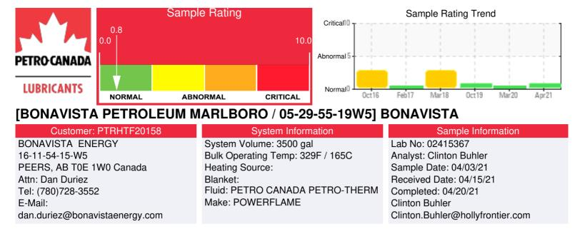
Recommendation: Sample results indicate that the fluid is in suitable condition for continued service. 90% distillation is slightly elevated as is solids content which can be associated to small amounts of fluid oxidation. Please ensure that blanket gas is being used in the expansion tank head space (2-3 psi ideal).Please re-sample in 12 months
