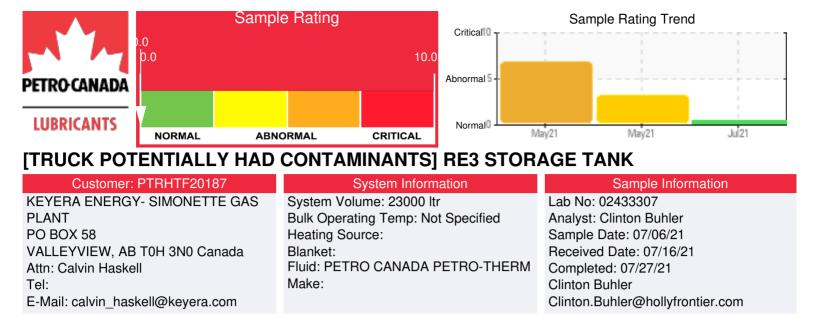
Recommendation: RE3 Tank re-sample results indicate that the fluid is not as contaminated as the initial samples from the tank trucks indicated. Please ensure that the fluid is kept cool, clean and dry while in storage
