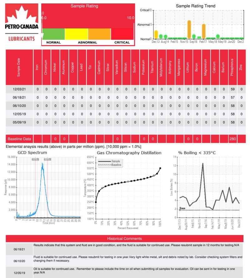
Oil is suitable for continued use. Please re-submit sample in 1 year. Acid number is normal, but has risen since the last sample, monitor at next test interval. Very light debris is noted by the lab.
