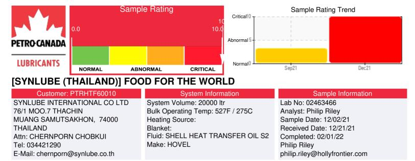
Recommendation: Not familiar with the chemistry of the Shell product. However, water level is extremely high and needs to be removed. SOurce of water ingress should be identified and rectified. Longer term I would expect the water to cause operational issues, acid increase, oxidation and corrosion within the system. Recommend an oil change, clean, flush and refill with CALFLO AF (most likely) but would discuss system conditions to best scope out product
