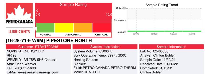
Recommendation: Sample results indicate the fluid is in suitable condition for continued service. Please re-sample in 12 months
