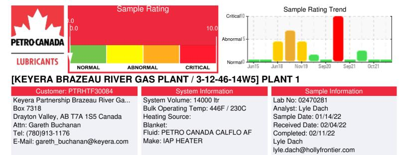
Recommendation: Sample results indicate that the fluid is in suitable condition for continued service. Resample in 12 months
