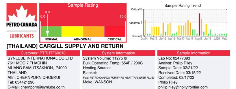
Recommendation: With exception of the COC Flash Point that is marginally low, all other parameters remain within acceptable limits. Please re-sample at normal frequency, oil if fit for further use
