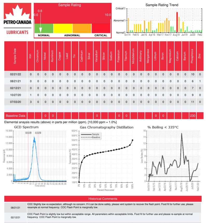
Flash Point marginally low and some evidence of light end fluid cracking that would create low boiling point products to explain that. If the system can be safely 10/27/20 vented then please look to do this. All other parameters are as expected and fluid fit for further use. Please re-sample at normal frequency COC Flash Point is marginally low.
