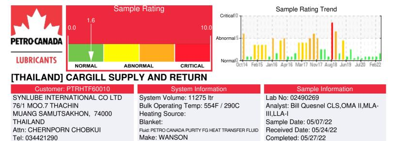
Recommendation: Flash point has decreased. Recommend that you vent the expansion tank to reduce low boilers. Resample at next interval to monitor.
