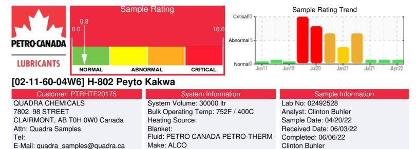
Recommendation: Sample results indicate that the fluid is in suitable condition for continued service. Low boiling vapor content has increased to 2.5%; this along with slightly reduced fluid viscosity and flash point may be associated with thermal degradation or possible mixing with process fluids. Please vent off low boiling vapors from expansion tank and re-sample in 6 months.
