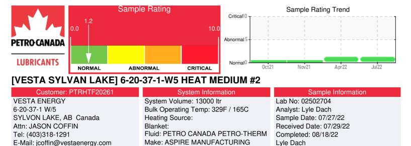
Recommendation: Fluid acid number is up slightly higher but the fluid PH is 7.24, fluid PH is neutral and would not be a concern to the system. Ensure the blanket gas is working but overall the fluid is in good condition for continued service. Resample in 6 months.
