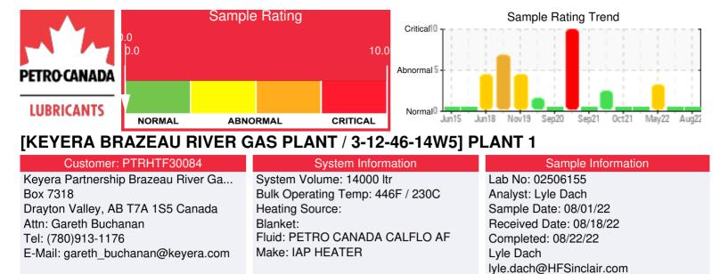
Recommendation: Fluid is in very good condition and is suitable for continued service. Fluids iPH is 6.54 and acid number is very low at 0.07. Resample in 12 months.
