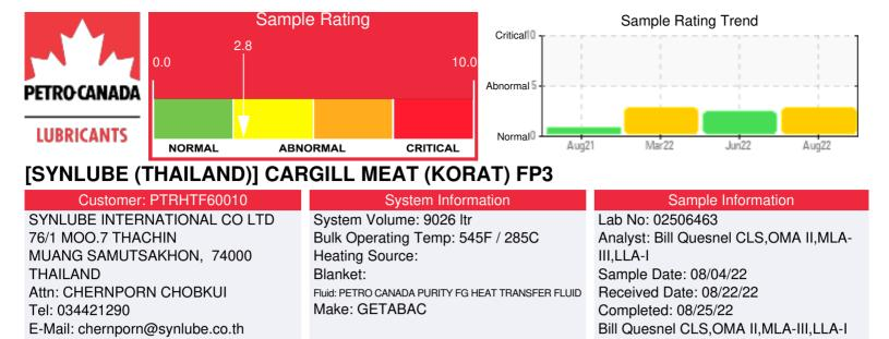
Recommendation: If venting was carried out, the flash point has not been restored. Site was visited 14th June and oil change recommended including a clean and flush of the system. Continue to vent the expansion tank until an oil change is carried out. Resample to monitor in 3 months time.
