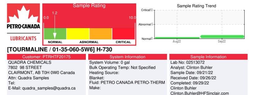
Recommendation: Sample results indicate symptoms related to either thermal degradation, mixing with process fluids and/or high blanket gas pressure: see reduced fluid viscosity and flash point and increased low boiler vapor content (4.45%). It is advised to perform regular venting of the expansion tank to remove the low boiler vapors which will help improve these parameters. Please contact Petro-Canada Technical Services to discuss further
