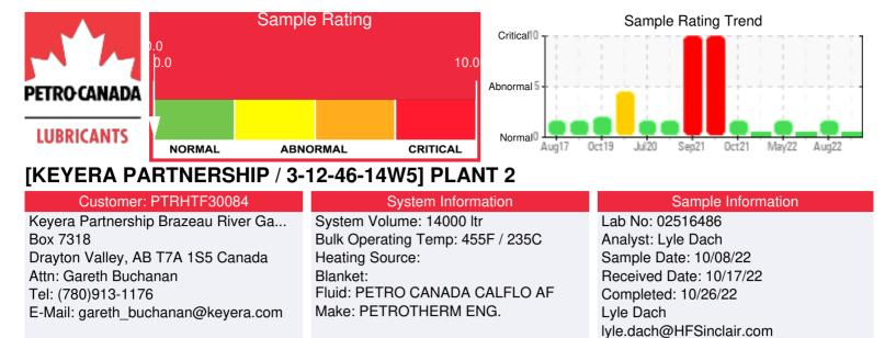
Recommendation: Sample results indicate that the fluid is in good condition and is suitable for continued service. Pentane insolubles are up slightly from the last sample. Resample in 12 months.
