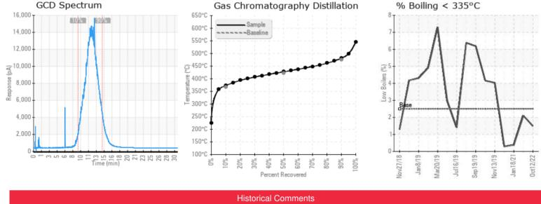
Sample results indicate that the fill of Calflo AF is in suitable condition for continued service. Please note slight increase in Fe content. Fluid parameters do not appear to indicate any proclivity towards corrosion. Please re-sample in 6 months
