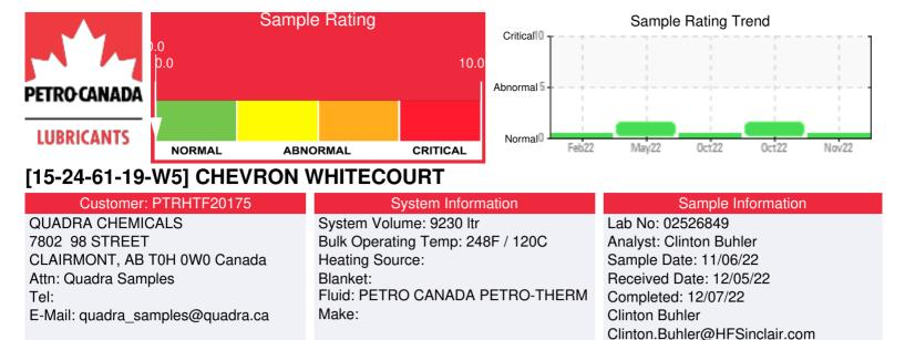
Recommendation: Sample results indicate the fluid is in suitable condition for continued service whereas the samples drawn October 6 and 18 2022 contained excessive water; so much that the fluid could not be analyzed. Please re-sample in 3 months to build a trend going forward. Please thoroughly purge sample port prior to collecting sample.
